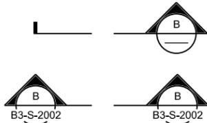
SECTION CALLOUT WHERE SECTION IS ON THE SAME SHEET AND CUT EXTENDS TO A FIXED LIMIT
